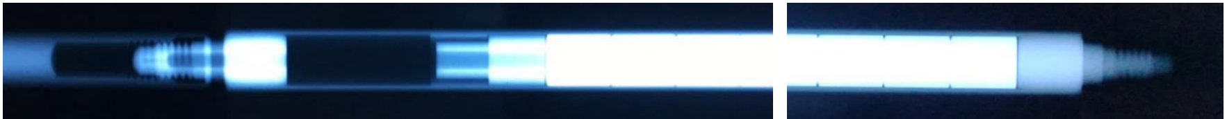
X-ray image of U_3Si_2 fuel segment built for Byron LTR
