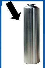
Both the glass matrix and compacted waste are encased in a standard "Universal Canister"
