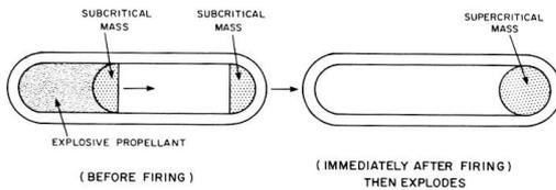
Figure 1.52. Principle of a gun-assembly nuclear device.
