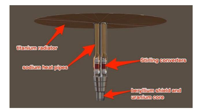
Image from Google: A diagram of a kilopower reactor
