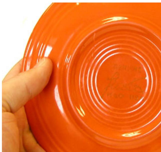
The red color was achieved by adding uranium oxide in the glaze - measurements have indicated that by weight, up to 14 % of the glaze might be uranium. How much glaze was employed per plate is unclear but it has been estimated that a single plate contains 4.5 grams of uranium (Buckley et al). Piesch et al estimated the glaze thickness at 0.2 mm.
