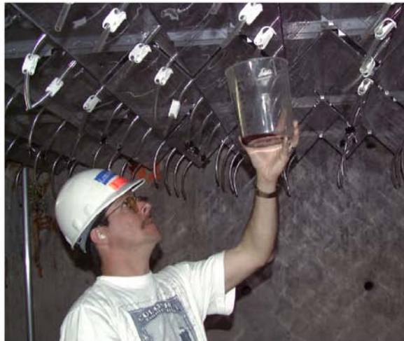
(b) Water Collection During a Drift Seepage Test
