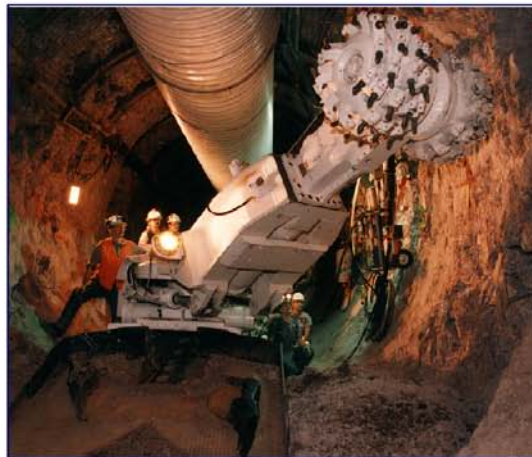
(b) Alpine Miner Excavating the Access Drift
